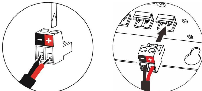
DarkFX Strip 1020 is wired to output terminal of DarkFX Drive 4 MKII. Each output terminal
