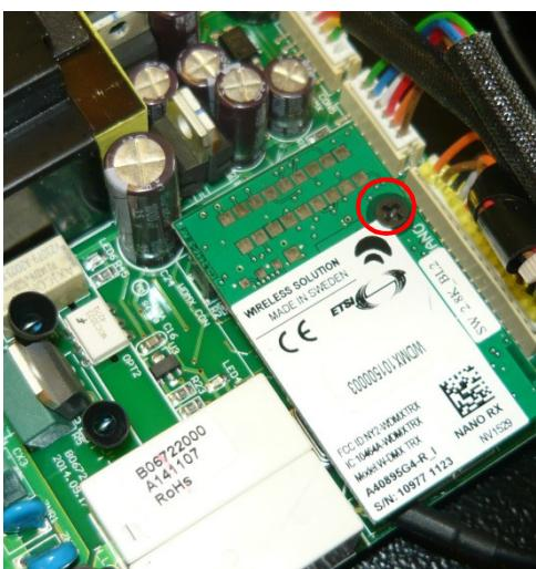
**Step 7.** Attach the W-DMX board to the main PCB and fix it with a screw. The installation of W-DMX antenna and W-DMX board is completed.
