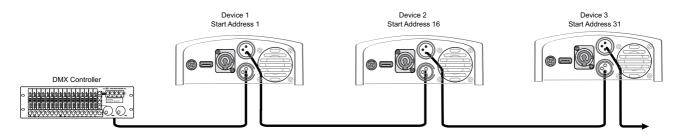
The wires must not come into contact with each other; otherwise the fixtures will not work at all, or will not work properly.
