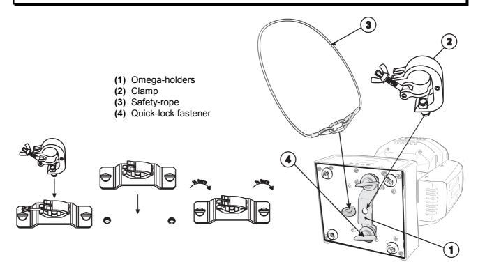
The device may be placed on the floor or fastened to a truss or similar rigging structure. The device must never be fixed swinging freely in the room.
