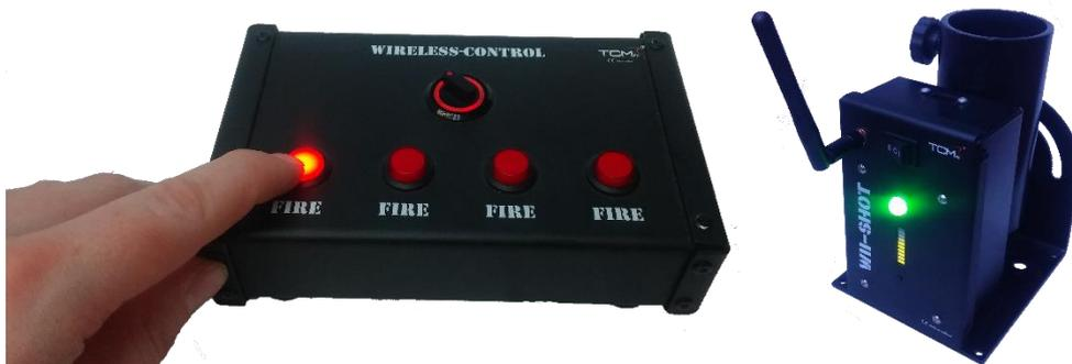
4. When ready to fire the confetti cartridge, turn the rotary switch to the right to arm the devices. The controller will automatically begin waking up the Wii-Shots, this takes about 4 seconds. After this you are ready to fire the Wii-Shot by pressing the previously assigned button.
