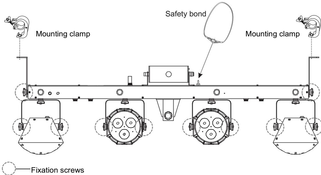
This product is designed for overhead rigging to a wall or ceiling with the mounting brackets. If necessary, it can also be fastened to a truss using appropriate clamps.
