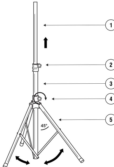
**Pull out the legs** – Loosen the safety screw (4) of the legs (5). Pull out the legs. Lock this position with the safety screw.
